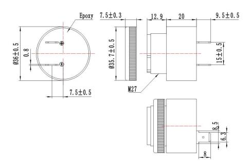
Unit: mm Tolerance: ±0.5mm Except Specified
