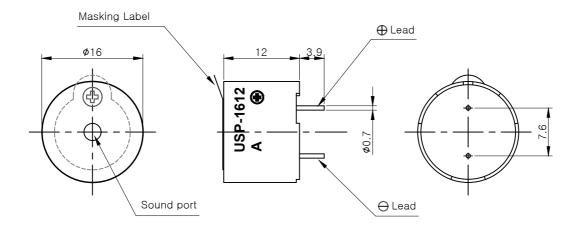
Tolerance: ±0.5mm Unit: mm Housing Material: Noryl(SE1-GFN2J)
