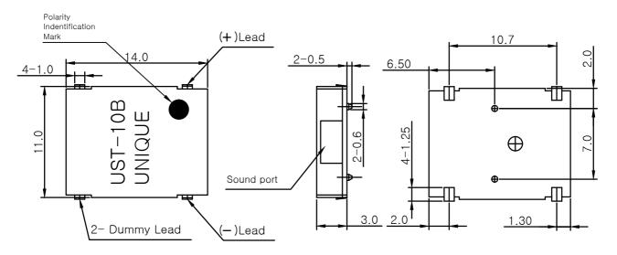
$\begin{array}{c} \text{UNIT: mm} \\ \text{TOLERANCE:} \pm 0.2 \\ \text{CASE MATERIAL: LCP(Black)} \end{array}$
