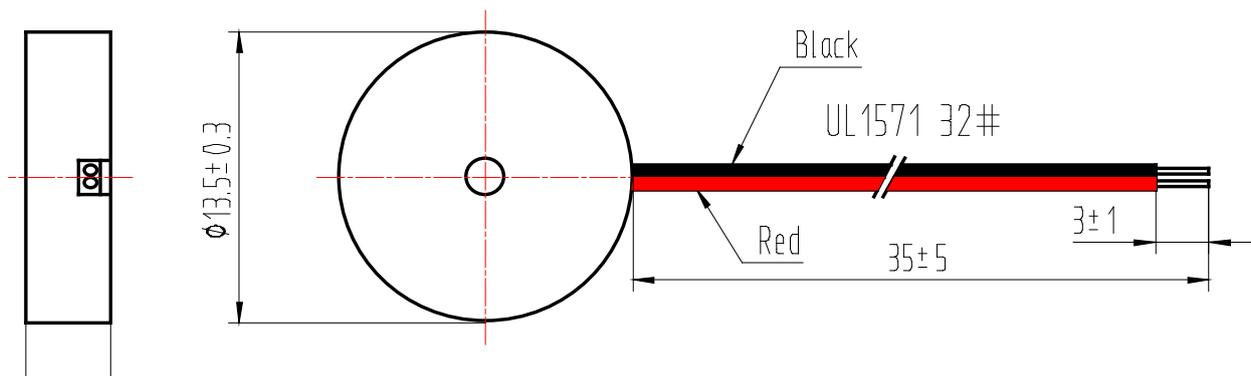
\*Unit: mm; Tolerance:  $\pm 0.5$ mm Except Specified
