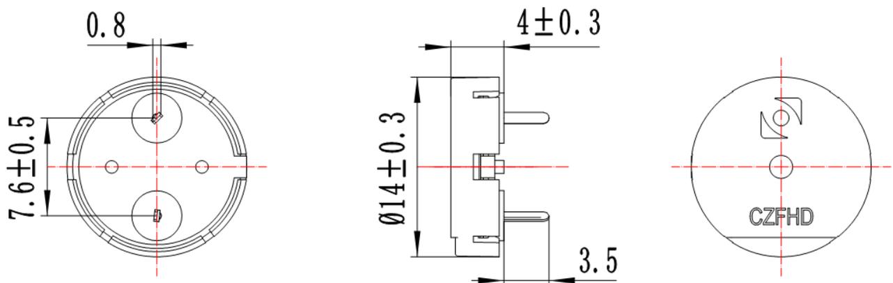
\*Unit: mm; Tolerance: ±0.5mm Except Specified
